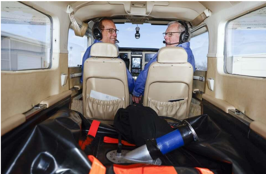
Peter Teahen (left) and John Ockenfels turn in their seats for a photo in the cockpit of the Cessna 210 Turbo Centurion airplane that they will fly around the world at the Iowa City Municipal Airport in Iowa City on March 27. The fuel bladder (bottom of the frame) when filled will come up to the lower edge of the side windows. Teahen and Ockenfels are taking off May 5 to fly around the world and raise money and awareness to help eradicate polio. The flight is aiming to raise $1 million for Rotary International's campaign to end polio. (Jim Slosiarek/The Gazette) JIM SLOSIAREK
